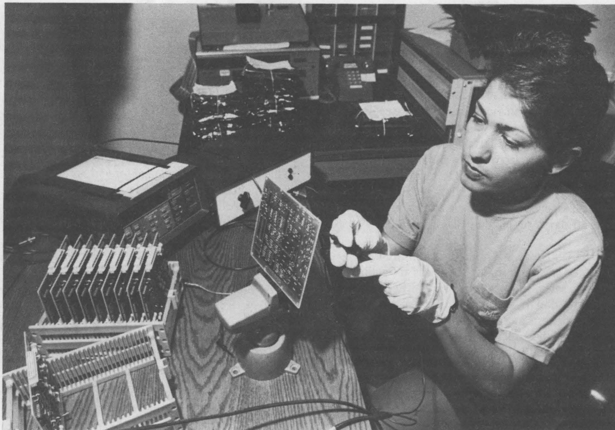
MARIA ARMENDARIZ (6613) tests operation of printed circuit boards after they have been subjected to environmental extremes such as humidity and heat. Her work is part of a cooperative research project between Sandia and Motorola. (Photo by Mark Poulsen, 3162)
